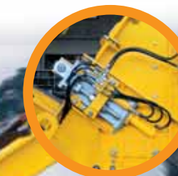
Impact arm hydraulically adjustable with integrated release system
